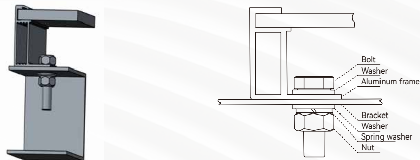
Figure 5 Bolt Installation of Mono-facial Modules
